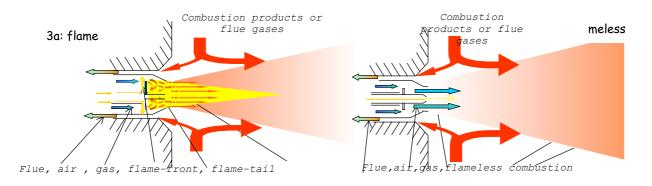
Figure 3 High velocity burner: flame and flameless mode
