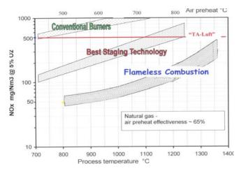
Figure 2 NOx from high temperature furnaces
